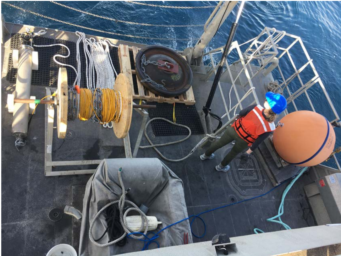
Staging of the CINMS NRS on R/V Shearwater. The hydrophone is the gray cylinder shown on the far left, line and cable are shown in between the hydrophone and the mooring anchor (old railroad wheel), and Nancy Foster Scholar Samara Haver is between the anchor and the sub-surface orange buoy that will sit highest in the water column.
